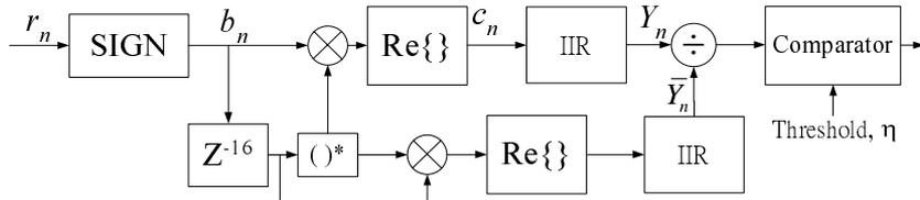
Fig. 3. The block diagram of the third signal detection algorithm.
