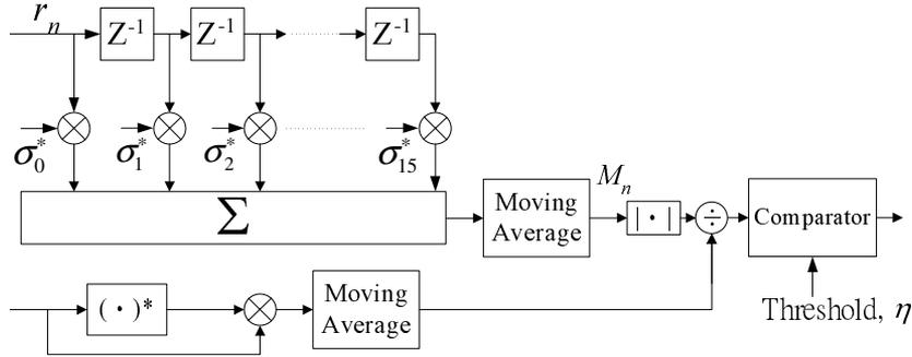
Fig. 2. The block diagram of the second signal detection algorithm.
