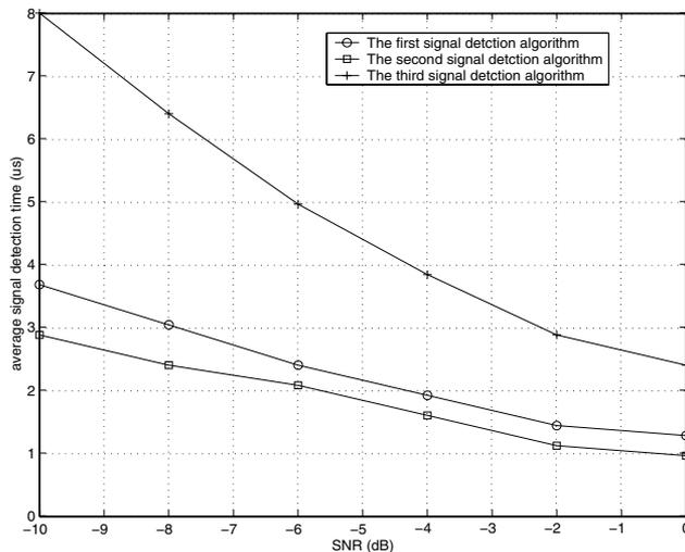
Fig. 5. Comparison of average signal detection time of the three signal detection algorithms.
