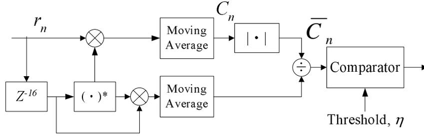
Fig. 1. The block diagram of the first signal detection algorithm.
