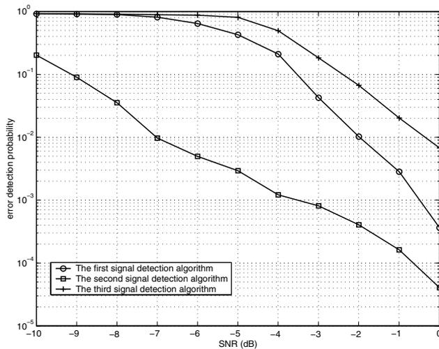
Fig. 4. Comparison of error detection probability of the three signal detection algorithms.
